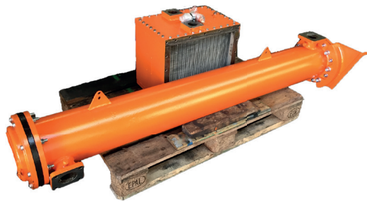
Overhauling of an inter cooler and oil cooler (shell & tube), painted in customers colors.
